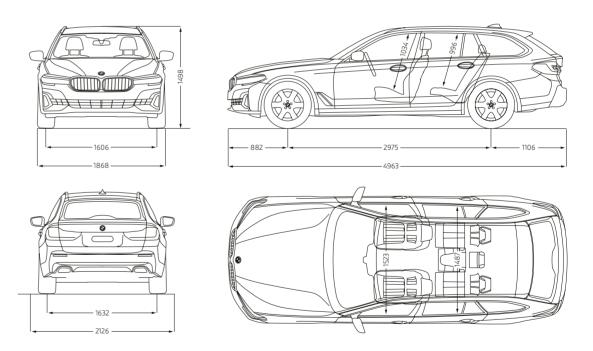
All dimensions in the technical drawing are given in millimetres.
