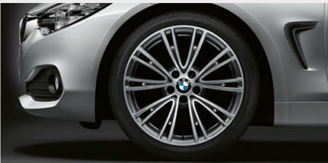
□ 19" light alloy wheels V-spoke style 626 I with mixed tyres, front 8J x 19 with 225/40 R19 tyres, rear 8.5J x 19 with 255/35 R19 tyres.
