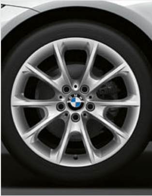
□ 18" light alloy wheels V-spoke style 398 with mixed tyres 2 , front 8J x 18 with 225/45 R18 tyres, rear 8.5J x 18 with 255/40 R18 tyres.
